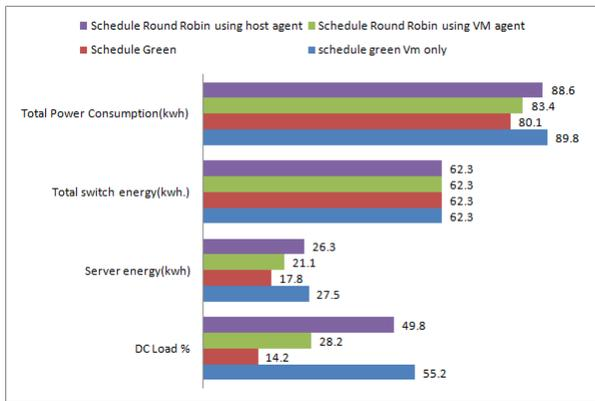
Figure 5.8: Power Consumption in Power Blade Energy Model
